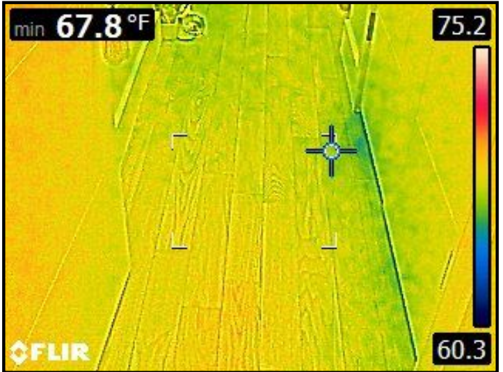
Infrared imaging of floor board separation point. No indication of water entry within the area. Separation caused by improper installation.
