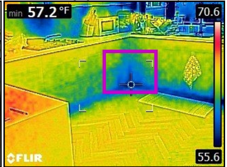
Infrared imaging of severe draft entry point.
