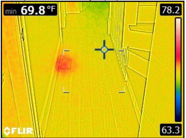
Infrared imaging of floor board separation point. No indication of water entry within the area. Separation caused by improper installation.
