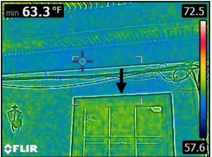
Infrared imaging of water cascading down through rear facade and backflowing into the internal wall/ceiling area.
