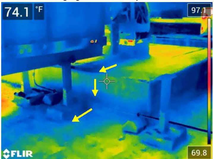
Infrared imaging of water entering through HVAC duct entry point into the roof membrane system and cascading down into the wall areas below.
