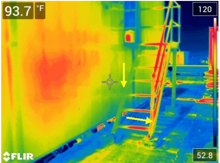
Infrared imaging of water entering through the bulkhead wall panels around the door baseplate and window, cascading down and depositing into the ceiling areas below.
