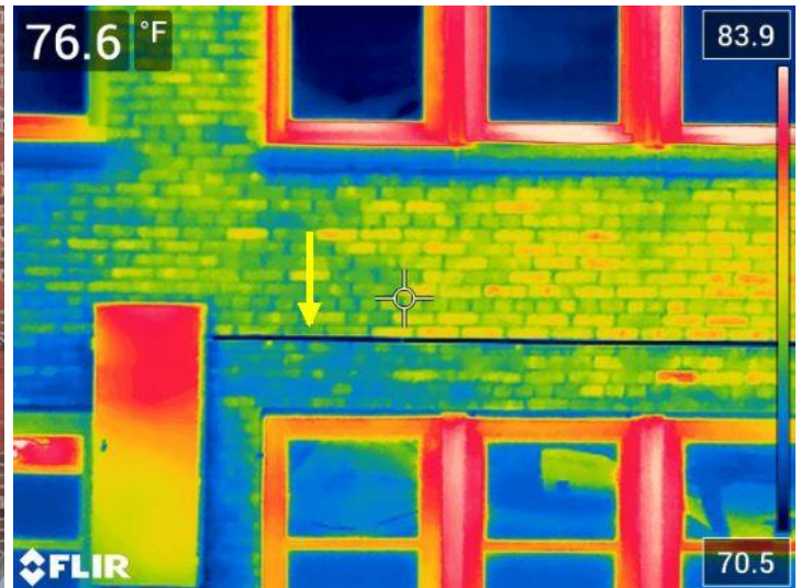
Infrared imaging of water entering through the window sill and brick facade areas, cascading down and depositing into the internal wall areas below.
